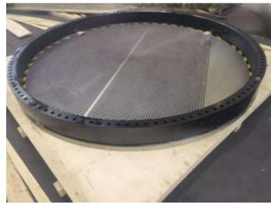
Flange &Tubesheet For Heat exchangers
